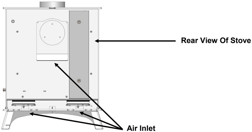
**NOTE : DO NOT COVER OR PARTIALLY OBSTRUCT THE AIR INLET OPENINGS FOR THE APPLIANCE.**
